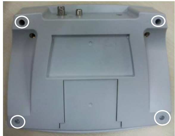
Figure 2-1. Screws (marked with white circles) that secure the housing.
